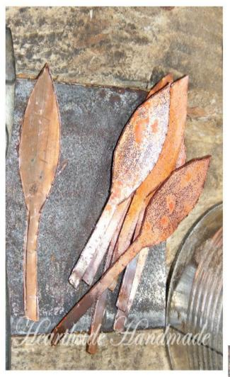
So the leaves were cut out, but still not thin enough for shaping. They were smaller pieces of copper now and could be more easily heated with just a propane torch. On the left, you see one leaf before torching and a pile of leaves after torching.
