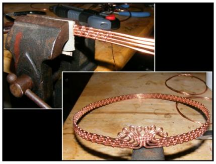
All that was left of construction was making the wire loops by the tail ends and mounting the whole thing on the band. Once done with construction, I made a paper cover for the eye, then sprayed the metal down with enamel.
